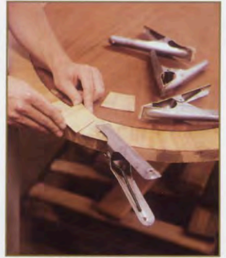
Exotic wood banding being applied
